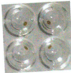
Fig. 2: MagSi-beads collected with MM-Separator M96 in 4 wells of a 96-well U-bottom microplate.
