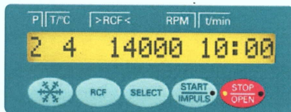
Control panel of the cooled UNIVERSAL 320 R
