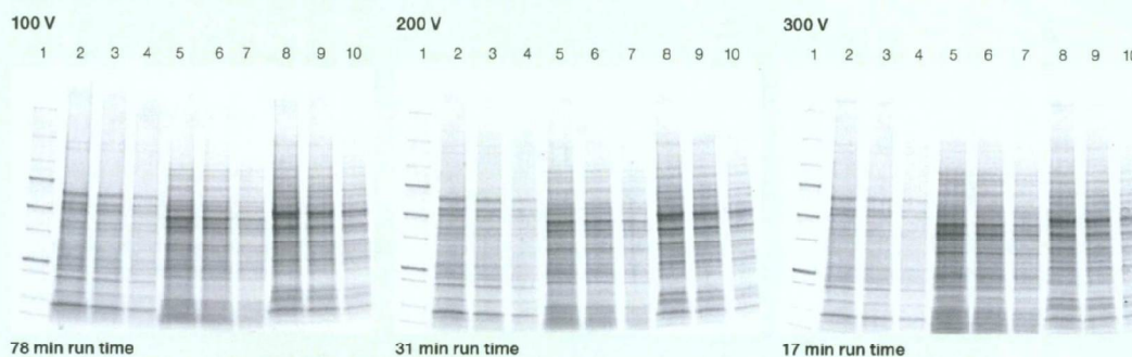
Fig. 4. 4–15% Mini-PROTEAN TGX Gels run at various voltages. Gels were loaded as follows: lane 1, Precision Plus Protein Unstained Standards; lanes 2–4, mouse liver; lanes 5–7, E. coli ; lanes 8–10, mouse brain.
