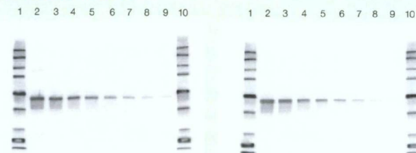
Fig. 2. Precision Plus Protein™ WesternC™ Standards and dilution series of a 51 kD protein tagged with GST detected by chemiluminescent western blot. E. coli lysate containing an overexpressed protein tagged with GST was electrophoresed on a 4–20% Mini-PROTEAN TGX Gel and blotted using the Mini-PROTEAN Tetra Blotting Core onto an Immobilon-P™ PVDF Membrane. The blot was then developed using the Immobilon-Star™ WesternC™ Chemiluminescent Kit and the image was acquired on the ChemiDoc™ XRS Imaging System. Lanes 1 and 10, Precision Plus Protein WesternC Standards; lanes 2–9, 51 kD protein tagged with GST 1,000, 500, 250, 125, 62.5, 31.3, 15.6, 7.8 ng, respectively.
